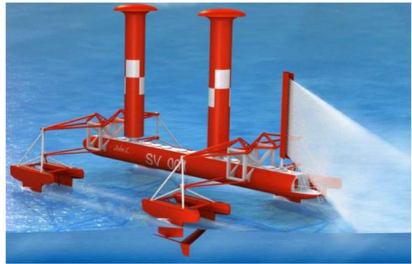
An artist's impression of the 2021 spray vessel. At full power of 300 kW from the wind they would release  $10^{17}$  drops a second.
